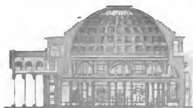
Fig. 377.—Section of the Pantheon. (Baumeister.)
